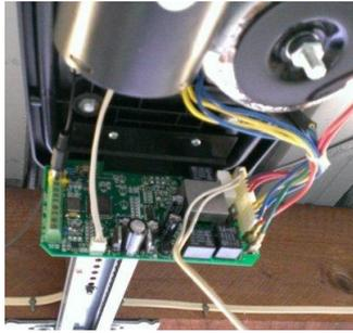
2. Hook up three wire receiver into Green terminals on the control board.
