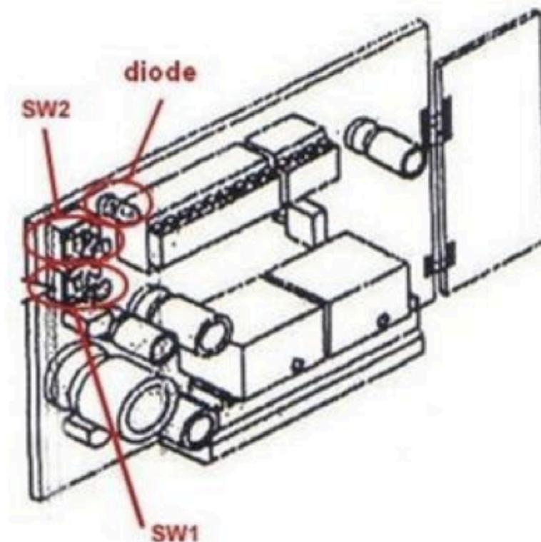
1. Open your motor, and try and find the receiver. If your receiver is in a case, then remove the casing. *You are trying to find something that looks like a control board*
