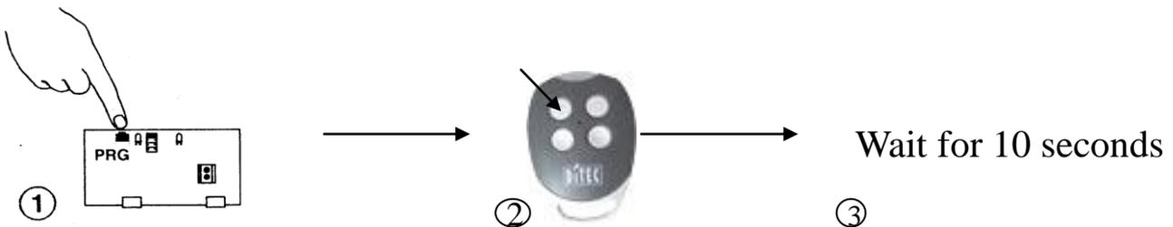
Press the black program button inside the control box (can be opened by removing the cover) for 5 seconds
