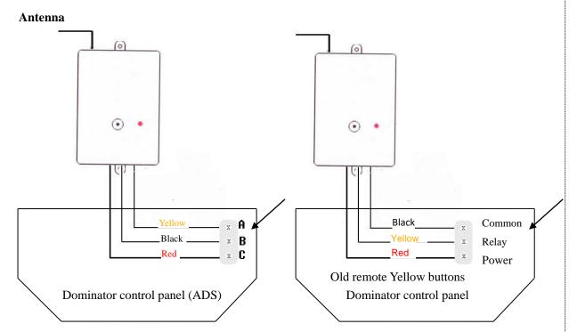
Dominator openers come two types of terminals A (START), B (GND), C (+24V) &
