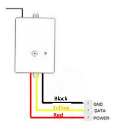
Note: the order of the wires connecting is different.
