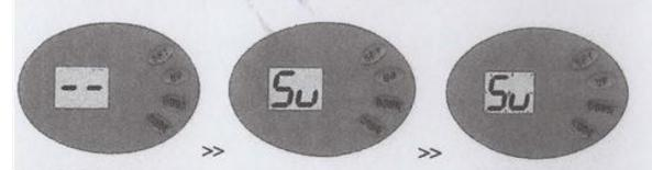
Press CODE, it displays "Su", press a button on the transmitter, then release and press the same button again, "Su" flashes, then it displays "= = " to show setting is complete.
