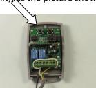
As the arrow pointing, the S1 (program) button is inside the receiver, then you can do the programming.
