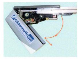
2. Remove the GTS cover by pulling in the directions of arrows as shown in the figure
