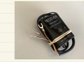
Red wire of the receiver hooks up to 24V terminal on the drive unit.
