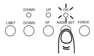
2. Press any button on the transmitter within 30 seconds.
