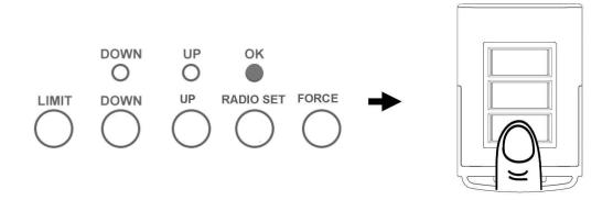
3. "OK" LED flashes once and operator beeps twice, acknowledging the transmitter is set.
