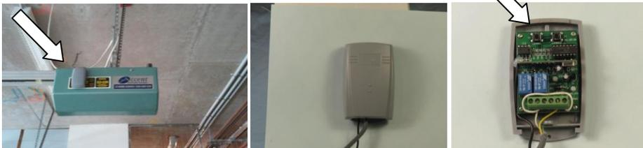
As the arrow pointing, the S1 (program) button is inside the receiver, then you can do the programming.
