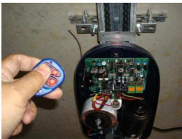
For **main entry door** of block unit, the S1 (LRN program) button is usually located in the stand along receiver ( it can be found near the drive unit), as the picture shown below:
