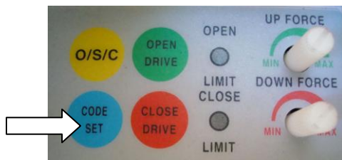
Fig1. GDO2,GDO4 control panel
