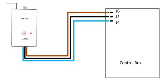
3. After open it, you can see there are 3 wires connected to 3 terminals on the control board (the pointed position on the photo). Disconnect the existing 3 wires, and connect the 3 wires of the MK receiver to the terminals.
